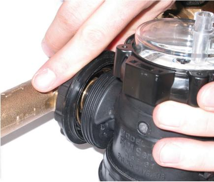
4. Hand-tighten Locking Nut by keeping the Measuring Unit vertically in position.
