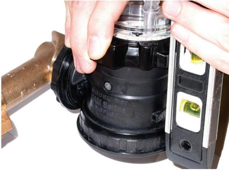
To loosen the locking nut, loosen clockwise.
