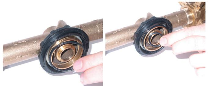
3. Position FAM Measuring Unit to Flow Tube; be sure the Measuring Unit is seated properly when mated with Flow Tube and that it is vertically level.
