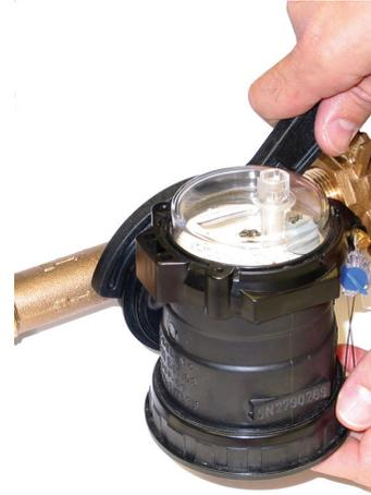
2. After installing and leveling the meter vertically, check to see if the Measuring unit is level horizontally. Level the Measuring Unit by loosening the locking nut clockwise, adjusting the Measuring Unit and tighten nut counter clockwise.
